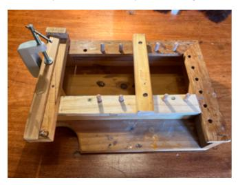
I adapted an old tabletop fly bench I made a few years ago and don't need anymore. This allows me to use various lengths of skin and stretch it tightly and hold it securely with some clamps.
