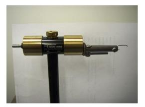
Precision ball bearing and heavy brass hubs enable the Nor-Vise to work like a spinning wheel allowing material such as dubbing or hackles to be spun onto the hook or onto the thread then onto the hook.
