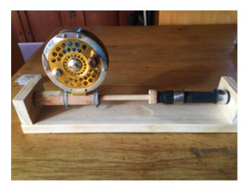
I reused a reel seat from a broken old spinning rod, a piece of broom handle, a couple of hose clips and a bit of leftover radiate pine to make the device.
