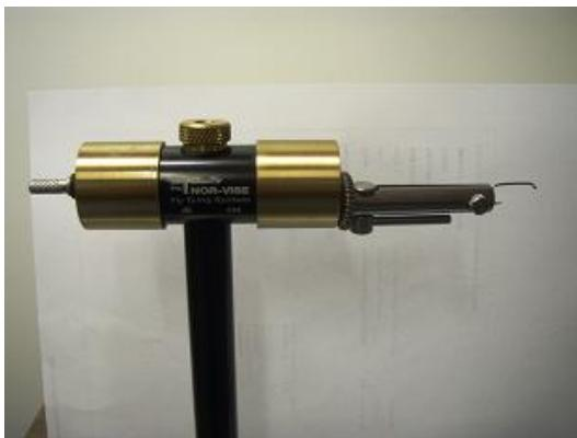
Precision ball bearing and heavy brass hubs enable the Nor-Vise to work like a spinning wheel allowing material such as dubbing or hackles to be
