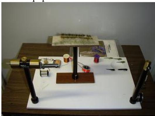
The Nor-Vise is an “in-line” rotary vise but the main difference with other rotary vises is that it spins (at speed) which allows some different tying techniques to be used.
