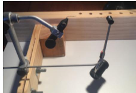
I have a special bobbin holder for my rotary vice. Its purpose is to hold the bobbin whilst I'm using the rotary function to wrap hackles and so on. It works really well
