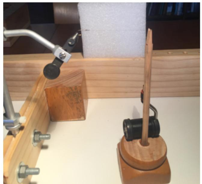
All it is is a simple base with a round dowel stuck (clumsily) in the middle. It works really well and I am now more likely to use the rotary function, which helps in accurate wraps, particularly with delicate hackles!
