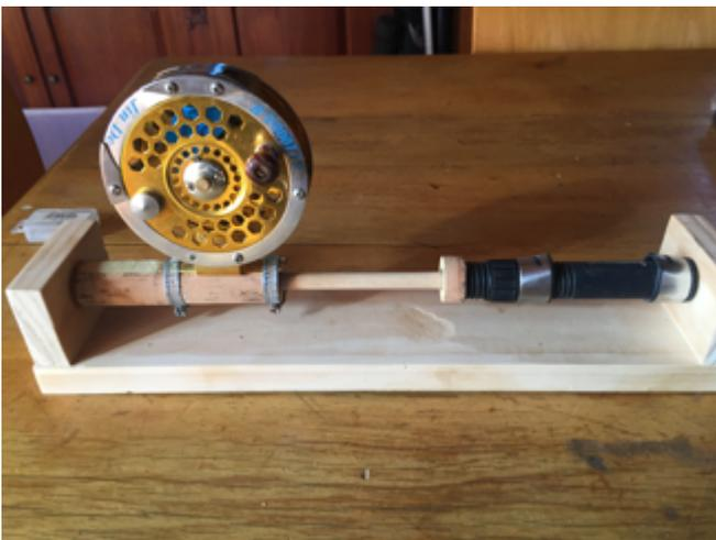
I reused a reel seat from a broken old spinning rod, a piece of broom handle, a couple of hose clips and a bit of leftover radiatae pine to make the device.
