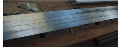
sadly mistaken - this is about a quarter of the way complete! With the two pieces bolted together tightly you pick up the file and proceed to flatten both sides of the form; many more than 10,000 strokes of the file.
