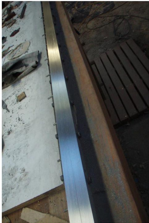
the block up and down the form, 20 thou is all that needs to be removed. Now I thought that 20 thou with 10,000 strokes to remove half a thou no problem go for it; it takes a lot less when removing the corners. Half a thou over the width of the form is a lot more cubic material than the corner. As a result I had to go back and reduce the top of the form down to get a correct depth at the tip end; worked on the third blister
