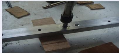
least the same. The directions tell me that first drill the primary hole for the thread to cut in the form, e.g. 8mm bolt I used a 6.5mm primary hole. This hole goes through both pieces. Before you move the form and do the second hole remove the 6.5mm bit and replace it with a 8mm bit. I found out that this really should be followed, the 8mm only goes through the first piece of the form to allow the shoulder bolt to slide unhindered.
